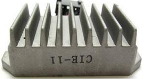
This regulator also in our tests did give 17V and does not support use without battery.
