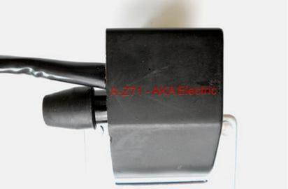
the above ighnition coil does not have the white ground wire as the original and also not the VAPE/PD labeling
